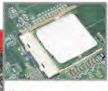
Note: Too much compound will decrease the performance of the CPU fan. The thickness should be between 1mm to 2mm.
